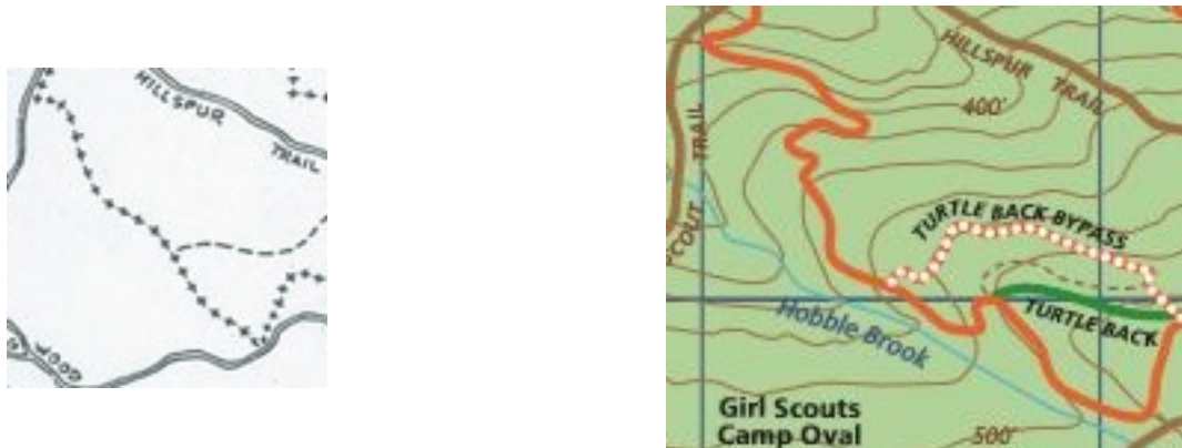
Figure 2.10: Reroute of upper Turtle Back trail avoiding fall line trail
